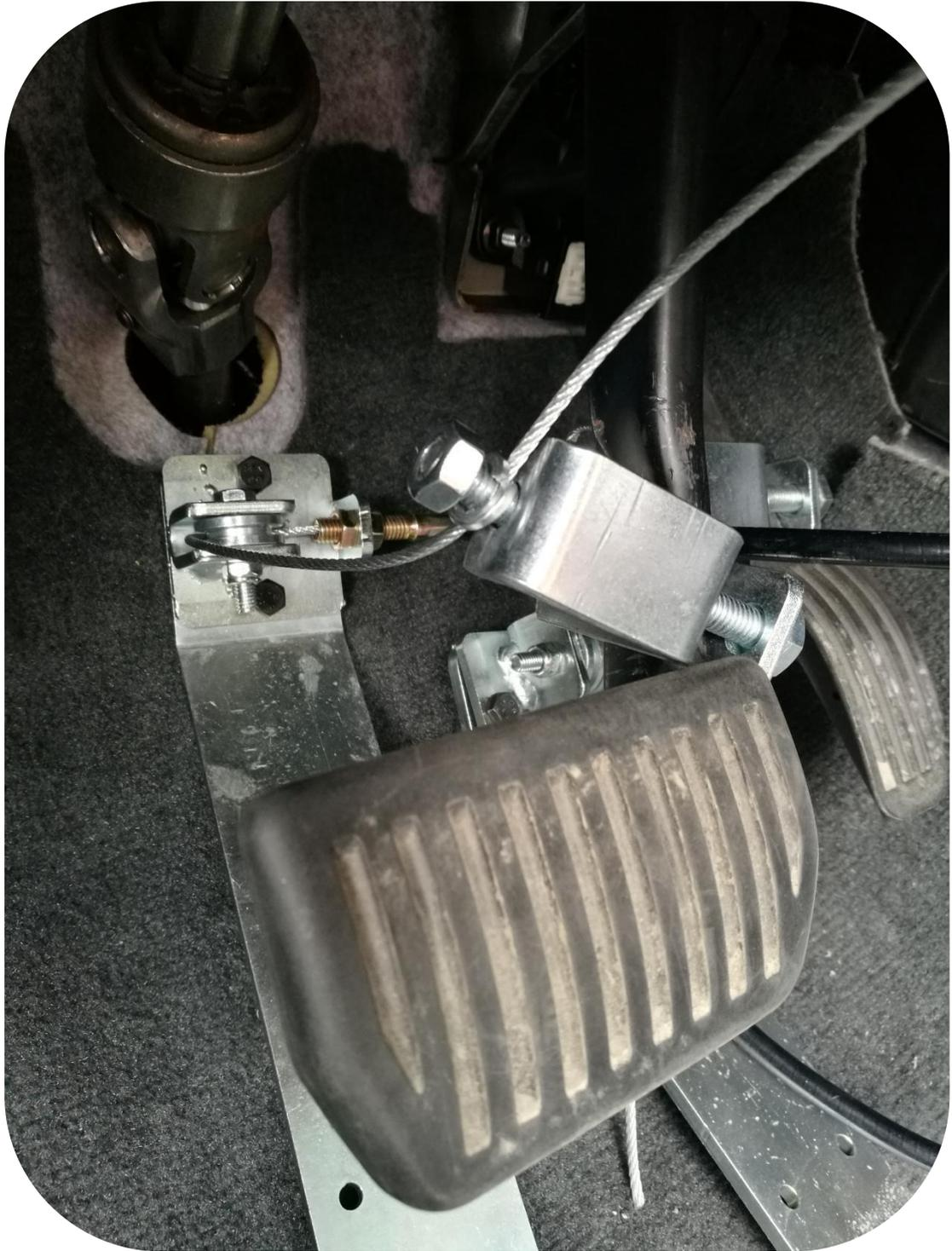
**Step 7:** Fix Chrome bar to car floor with pistol drill.
