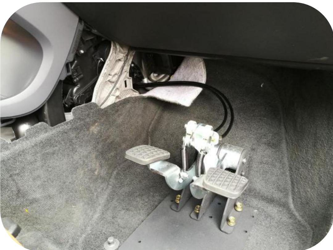
**Step 3 :** Pull out the cable, now you can see the cable in driver side.
