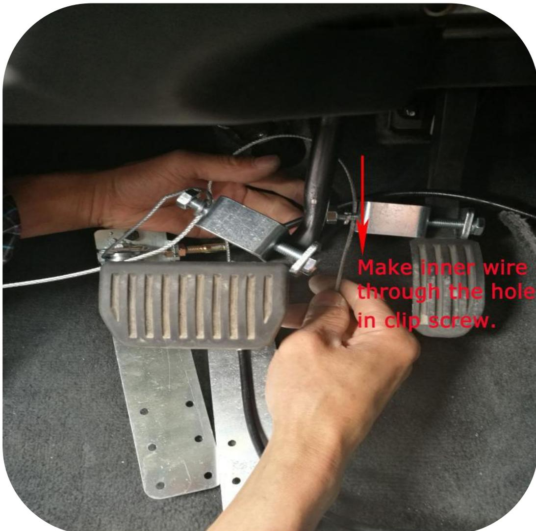
Make inner wire through the hole in clip screw.
