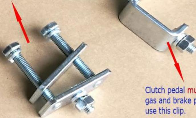
Clutch pedal **must** use this clip, gas and brake pedal could also use this clip.
